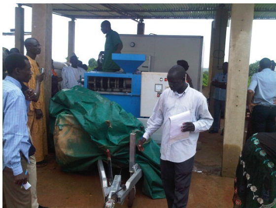
Figure 10: MaliBiocarburant's mobile press mounted on a trailer [D]
